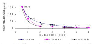
**Figure 3: Mixing speed and initial emulsion (15 min) in combine process** (500ml crude oil, 1.5% water, 1.5% buffer, 2ml enzyme at 40°C)
