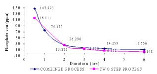
**Figure 4: Combined and two step Enzymatic degumming** (500ml oil, 1.5% buffer, 1ml enzyme, 1000rpm, at 40°C)
