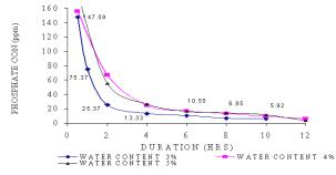
**Figure 1: Water amount in the enzymatic egumming of crude oil** (500ml crude oil, 1ml enzyme, normal mixing 1000rpm at 40°C)
